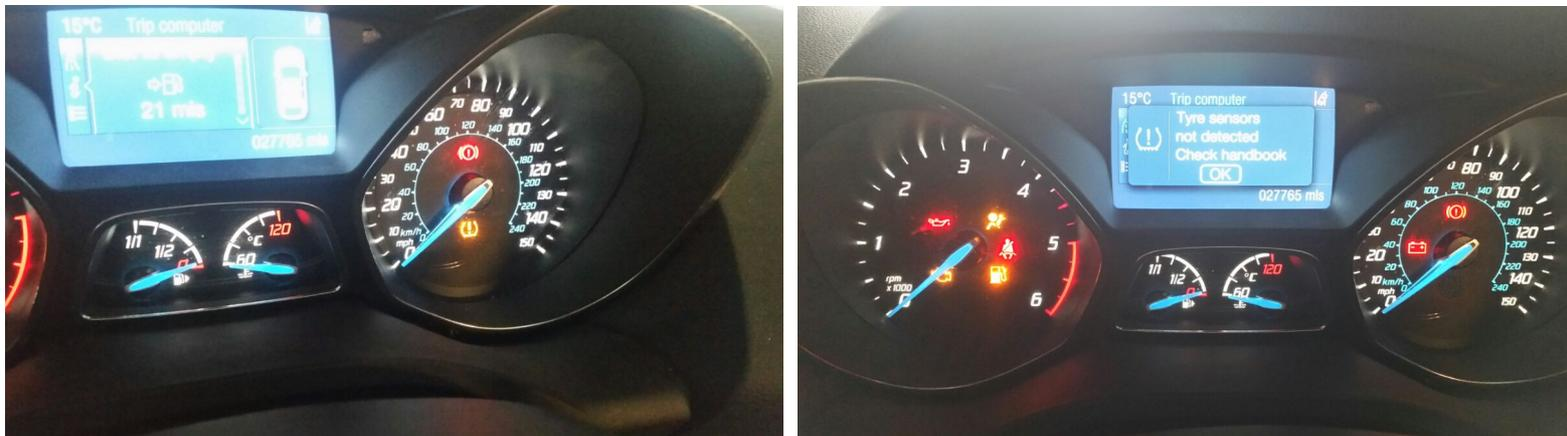
The issue does not affect the overall driveability of the car, but according to the European regulations, all cars must have these sensors. It is up to the owner of the vehicle whether he will fix the error with replacing the sensors or put tyres without the sensors and clearing the warning.
